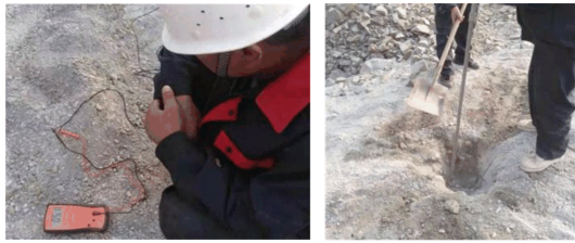
a) 测量致裂管导线电阻 Measure the resistance of the cracker tube wire
